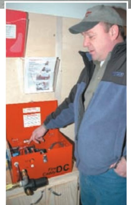
lake, creek, or to a tank in the back of a truck or on a trailer. The pumps run on a 5.5-hp motor, and both systems come with up to 300' of hose as well as 20' of suction hose. As well,
