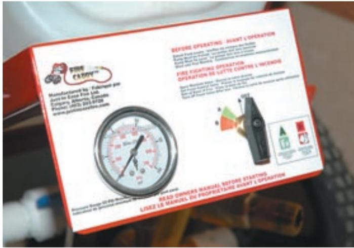
The system's pressure gauge tells the operator if the water pump is running the way it should.
